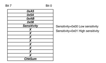
**RD\_RX\_SENSITIVITY** This command is sent to the TCM to retrieve the current radio sensitivity mode (HIGH or LOW). This information is sent via an INF\_RX\_ SENSITIVITY command.
